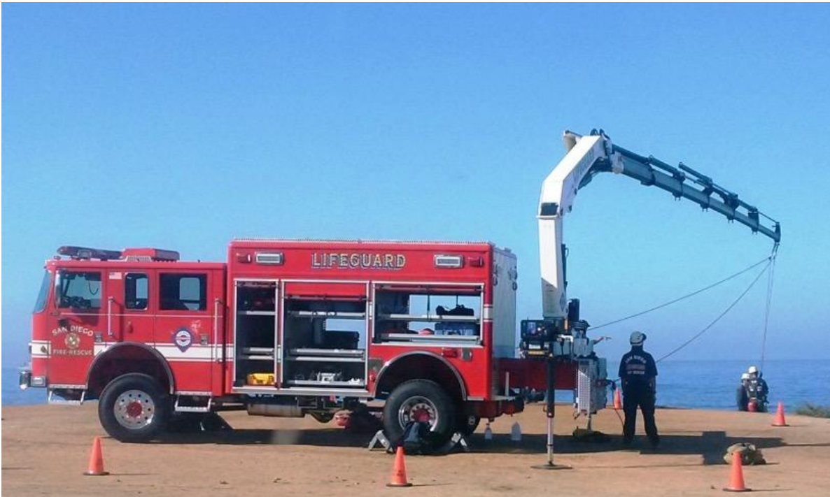
Lifeguard Rescue 44, which has a retractable boom, is a specialized truck for cliff and inland water rescues.
